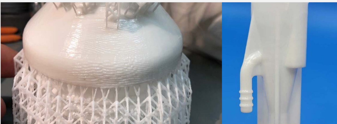
Difference between an under-cured part with wavy surface (left) vs correctly cured part with uniform glossy surface (right)
